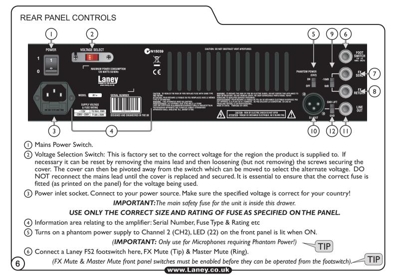
7) FX SEND: Mono jack socket for connection to the input of an external FX unit.
